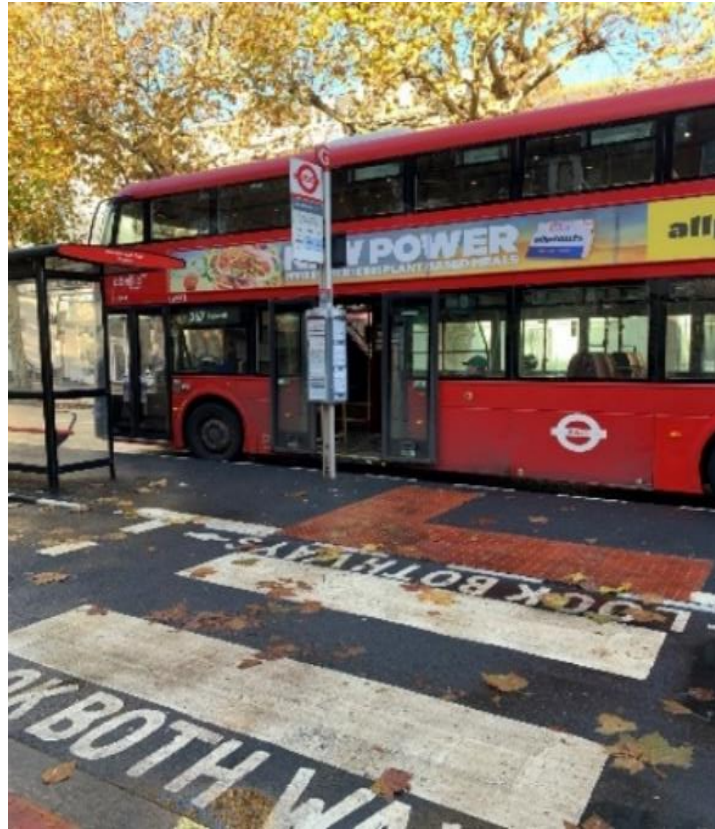
Figure 9: Bus stopping with its doors opening onto the bus pole and flag, creating an obstruction to those alighting. This is at Bus Stop G, Ravenscourt Park.
